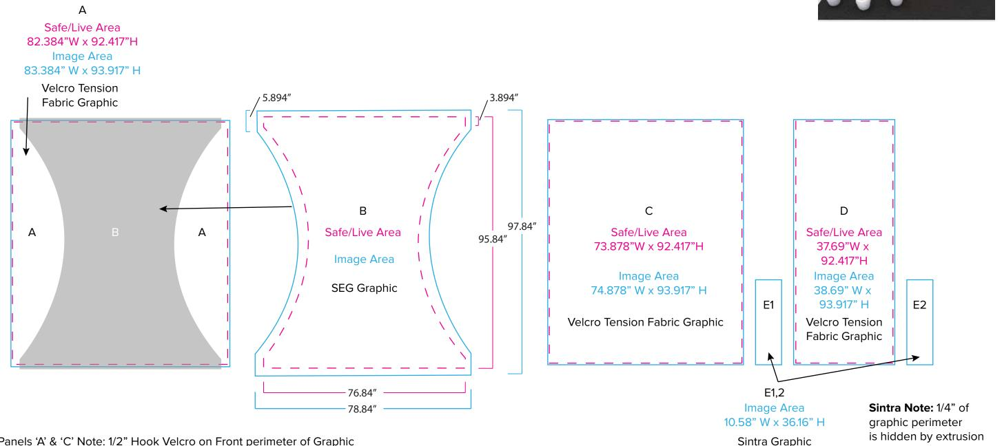
Panels 'A' & 'C' Note: 1/2" Hook Velcro on Front perimeter of Graphic
